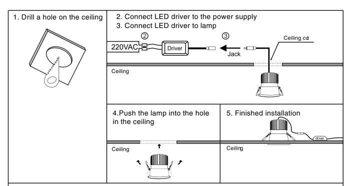
Note: - Disconnect the power supply before connecting the power
