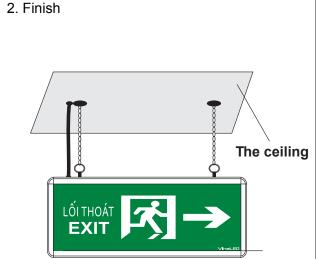
Note: Turn off the power, check the entire power system before installation
