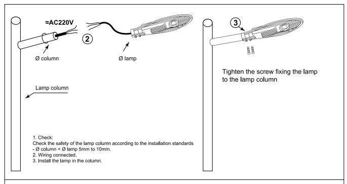
Note: - Disconnect the power supply before connecting the power - Need to activate the warranty before use. If not activated, the applicable time is the factory time.
