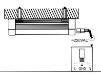
4. The power plug at both endsof the led tube is the same. Connect the led tube in series with the connector
