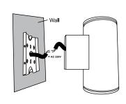
3. Connect the lamp body to the bracket. Then fix them with stainless steel screws
