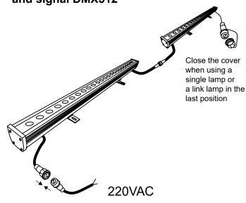
Note: - Disconnect the power supply before connecting the power
