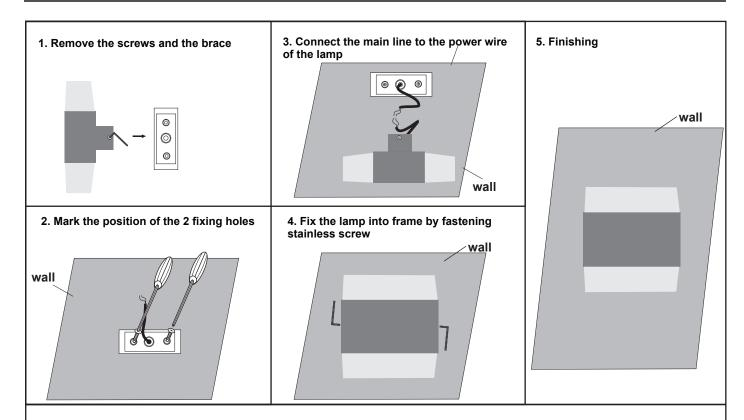
**Note** • Turn off the power at the circuit breaker and ensure that the power is off before wiring
