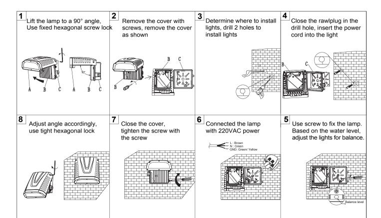
**Note:** Disconnect power, check safety of the entire electrical system before construction. Only installed by qualified electricians.
